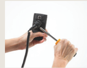
Holding merchandise vertically, pull down on handle to release sensor
