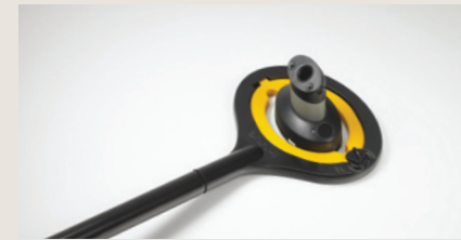
2. Rotate Removal Tool handle to remove
