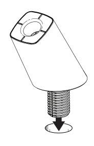
Below fixture: Fully tighten plastic nut onto stand.
