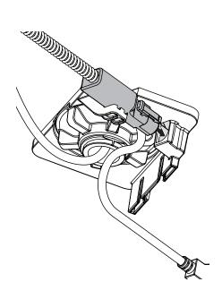
Plug power supply into sensor cable and outlet.
